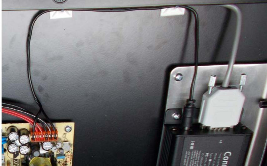
Figure 10. Connect Cable Assemblies
