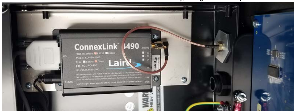
Figure 8. Mount ConnexLink Radio to Bracket
