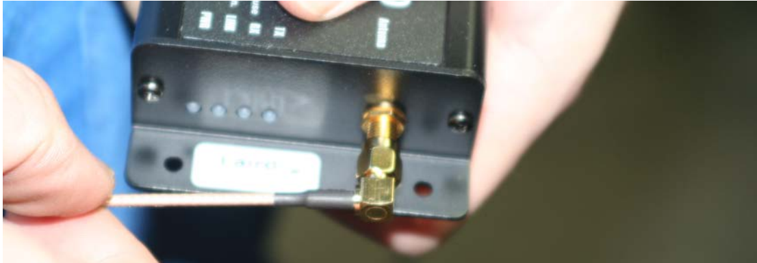
Figure 7. Attach Cable Extension Antenna to ConnexLink Wireless Radio
