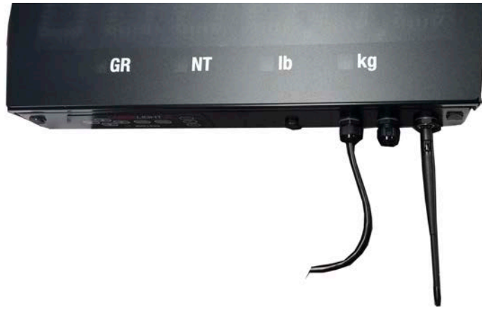
Figure 5. Thread Antenna onto LaserLight2
