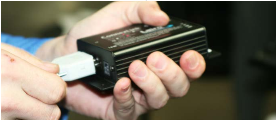
Figure 6. Plug 9-Pin Connector
