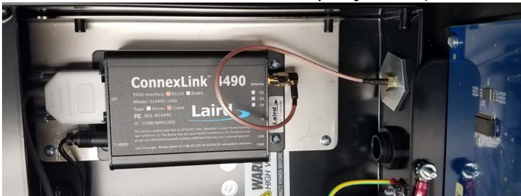
Figure 8. Mount ConnexLink Radio to Bracket
