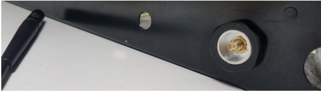
Figure 4. Thread Antenna Extension Cable Through
